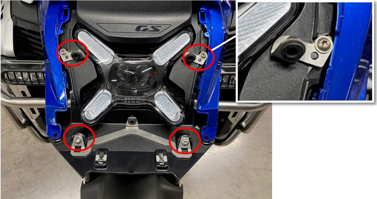
4x Schrauben befestigen / 4x tighten screws
