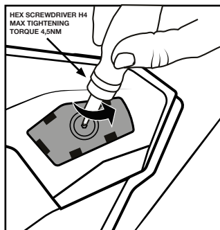
3 UNSCREW AND LIFT THE PEAK
