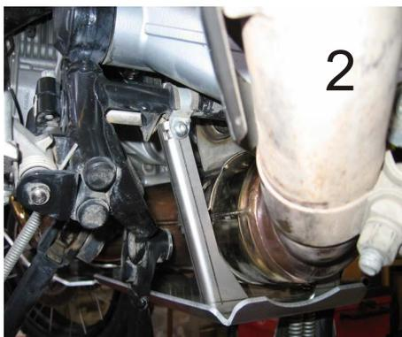
1.) Remove first the original BMW motor guard and exchange the original rubber-metal bolts with the ones supplied in the package. Be careful not to tear the stock bolts!
