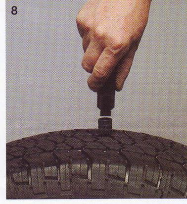
8 Screw loaded Plugger onto nozzle in tire
