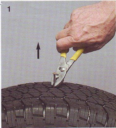
1 Locate puncture and remove damaging item
