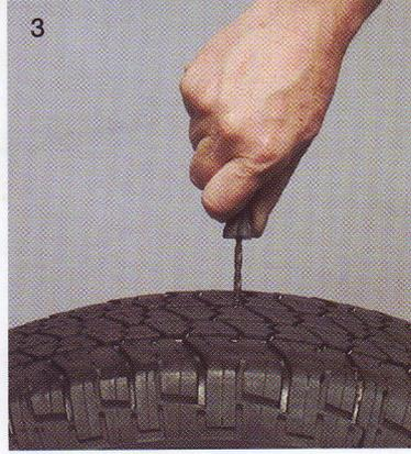
3 Thoroughly ream out hole with rasp tool
